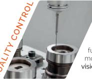
Quality department assures the steel dimensions of all the cavities and stacks. It also measures the final parts produced during the mould trials, providing you with the full dimensional report using the most advanced CMM and quick vision equipment.
